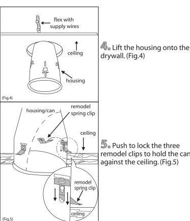
5° Push to lock the three remodel clips to hold the can against the ceiling. (Fig.5)
